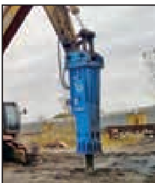
Hammer HS 15000, 15,500kg the largest rock breaker ever produced - SME Plant Sales.
