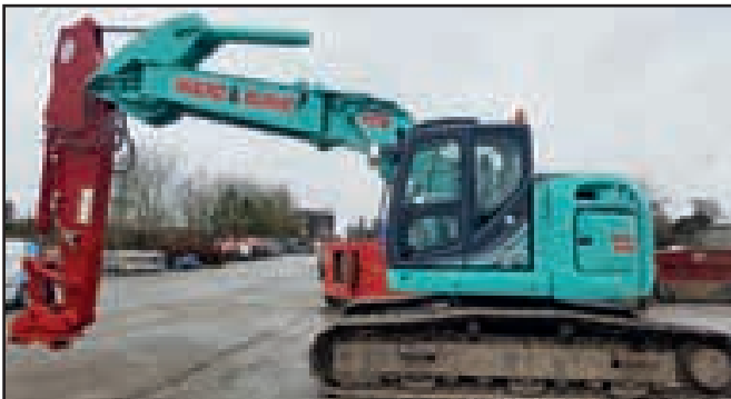
SK270SRLC-5 supplied by McSharry Bros and off-set boom fitted by Ward & Burke Construction Ltd., Co. Galway.
