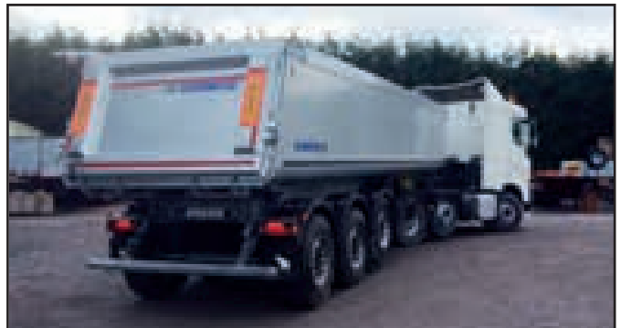
NEW Schmitz aluminium tipping trailer, rear steer axle, front lift axle, roll over cover, option of steel body also
