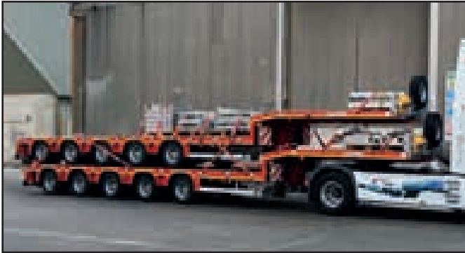
NEW Unused 5 axle Faymonville MAX step frame trailers, payload 65tons, extendable, option for hydraulic ramps.
