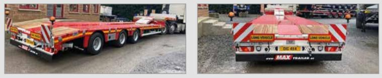
New Faymonville MAX100, 3 axle step frame extendable low loader, with out riggers, marker boards, two sets of aluminium ramps
