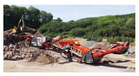
have the machine configured with fingers to scalp oversize, 100mm impact plate, onto 40mm tines, then a 12mm x 100mm slotted mesh on the lower deck to remove the the fines," says Russell.
