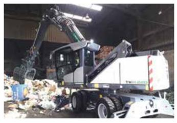
most obvious features are its unique long-reach boom, arm and 4-toothed grab attachment. Operationally, the TWH 220 has a reach of 10.4 metres, and comes fully designed and specified for the job it must do. Its hydraulically powered high-rise cab is designed and functions to ensure that the operator has perfect visibility within the worksite at all times.
