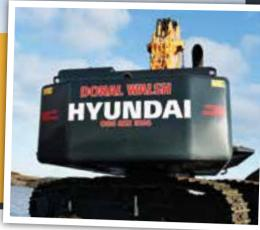
Donal Walsh and Whelan Plant Sales, the machine offers a maximum digging depth of 9.6 metres while yielding maximum reach at ground level of 14.43 metres.
