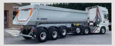
New Schmitz 8.2m Hardox Steel Body tipping trailer, roll over cover, steel galvanised chassis, choice of axles
