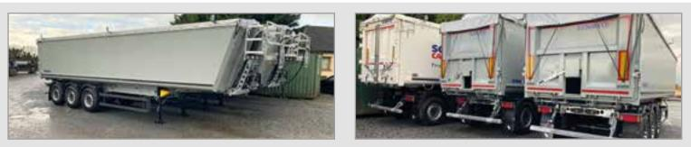
New Schmitz Alumimiun bulk tipping trailers, choice of size 64 cubic yard, 70 cubic yard, with grain hatch, sealed top hinged rear door, roll over cover, galvanised steel chassis
