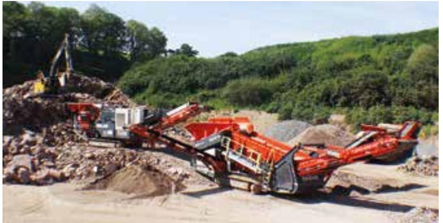
have the machine configured with fingers to scalp oversize, 100mm impact plate, onto 40mm tines, then a 12mm x 100mm slotted mesh on the lower deck to remove the the fines," says Russell.
