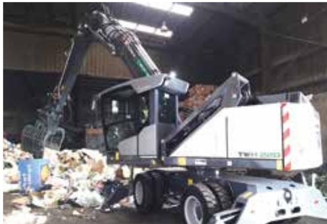
most obvious features are its unique long-reach boom, arm and 4-toothed grab attachment. Operationally, the TWH 220 has a reach of 10.4 metres, and comes fully designed and specified for the job it must do. Its hydraulically
