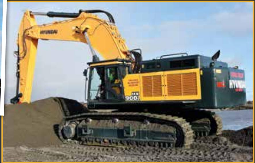
Donal Walsh and Whelan Plant Sales, the machine offers a maximum digging depth of 9.6 metres while yielding maximum reach at ground level of 14.43 metres.
