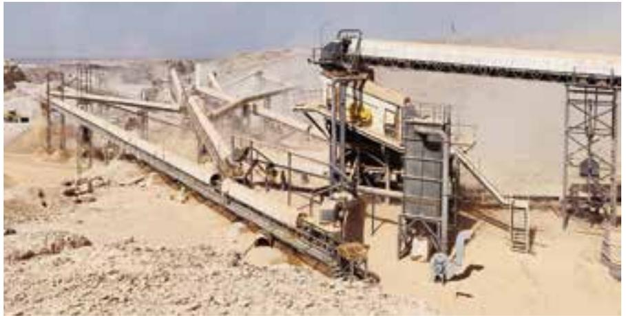
the impressive set up spans approximately 4,20,000 sq.mts and produces 20,000 Metric ton per day ranging from 0-5mm, 5-10mm, 10-20mm, 20-40mm, 40-80mm.
