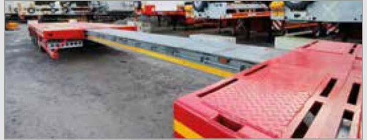
New Faymonville Multimax, 9ft wide, plus out riggers, extendable, two sets of aluminium hook on ramps, post sockets, two rear steer axles
