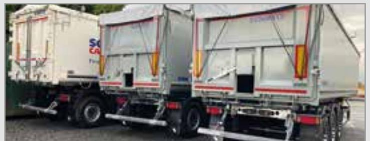
New Schmitz Aluminium bulk tipping trailers, choice of size 64 cubic yard, 70 cubic yard, with grain hatch, sealed top hinged rear door, roll over cover, galvanised steel chassis
