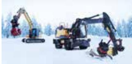
"The fully automatic quick coupler system brings a huge increase in efficiency, as excavator operators never have to leave the cab to switch between different hydraulic tools," says Sven-Roger Ekström. "At the same time, safety is significantly increased since no one needs to enter the risk zone around the machine during tool changes, and there are no concerns relating to dropped or uncontrolled movement of tools."
