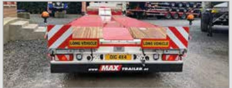
New Faymonville MAX100, 3 axle step frame extendable low loader, with out riggers, marker boards, two sets of aluminium ramps
