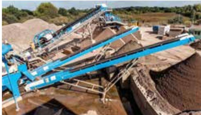
material by producing washed and graded recycled sand and aggregates including drainage stone, MOT Type 1 and 65F.
