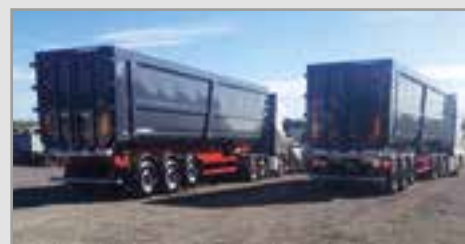
New Schmitz 80 cubic yard bulk scrap trailer, hardox steel body, barn doors with safety lock, front lift axle, very strong trailer with light tare weight, 8 tons, in stock ready to go.
