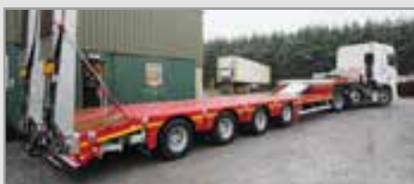
New Faymonville 4 axle step frame low loader, fixed bed, double flip ramps with hydraulic side shift, out riggers, marker boards, 48ton payload.
