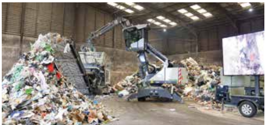
The new TDS 825 Slow Speed Shredder reducing bulky waste material with ease at RiverRidge, Maydown facility.
