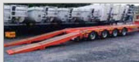
New Faymonville 4 axle 9ft wide, extendable, payload 60ton, double flip ramps, hydraulic legs under rear, out riggers, marker boards, ready to go.
