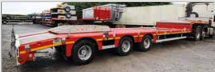
New 3 axle step frame low loader, extendable, with hook on aluminium loading ramps. 39ton payload, stake pockets and twistlock pockets.
