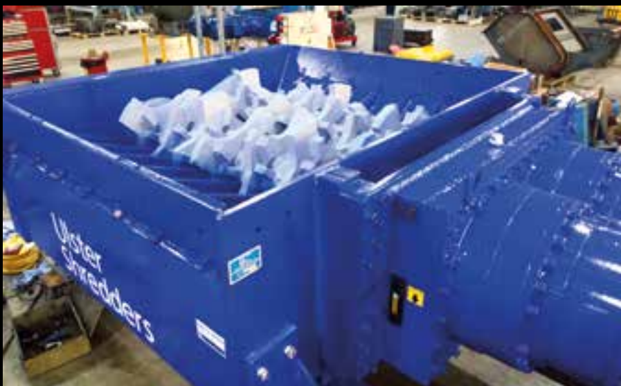
A special shredder designed for large diameter cardboard cores for Highlander nears completion in the Ulster Shredders factory.
