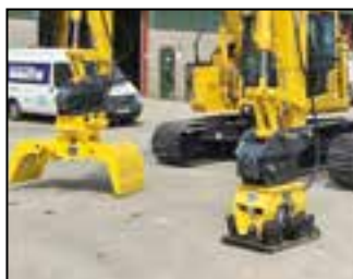
2 new PC138US-11 excavators c/w Epiroc Multi Grapples & Hydraulic Compactors supplied to CP Hire by WAC McCandless.
