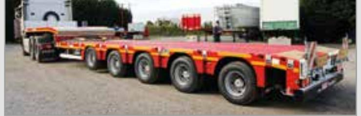
New Faymonville 5 axle step frame extendable low loader, 3 steeraxles, front lift axle, auto greaser, option on for hook on aluminium ramps or hydraulic ramps.
