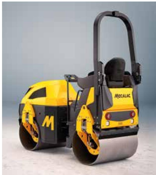
While most tandem rollers are manoeuvred using a steering wheel, the TV1200 has been re-imagined with a joystick design. With their back comfortably against the seat and right hand on the joystick, the driver has complete freedom to position their legs comfortably while keeping their eye on the work.
