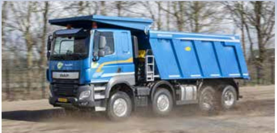
In addition to the existing 7.5, 8 and 9-tonne front axles, the new 10-tonne version in the CF and XF will be offered from the second half of this year. This is of particular interest for applications in the construction segment, where high front axle loads are commonplace.
