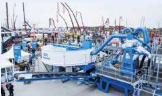
CDE has launched the Combo in a move set to revolutionise the wet processing industry; the world's first all-in-one wet processing plant encompasses five processes - feeding, sizing, sand washing, stockpiling and complete integrated water management which is a first for the industry and an important innovation to address a challenge
