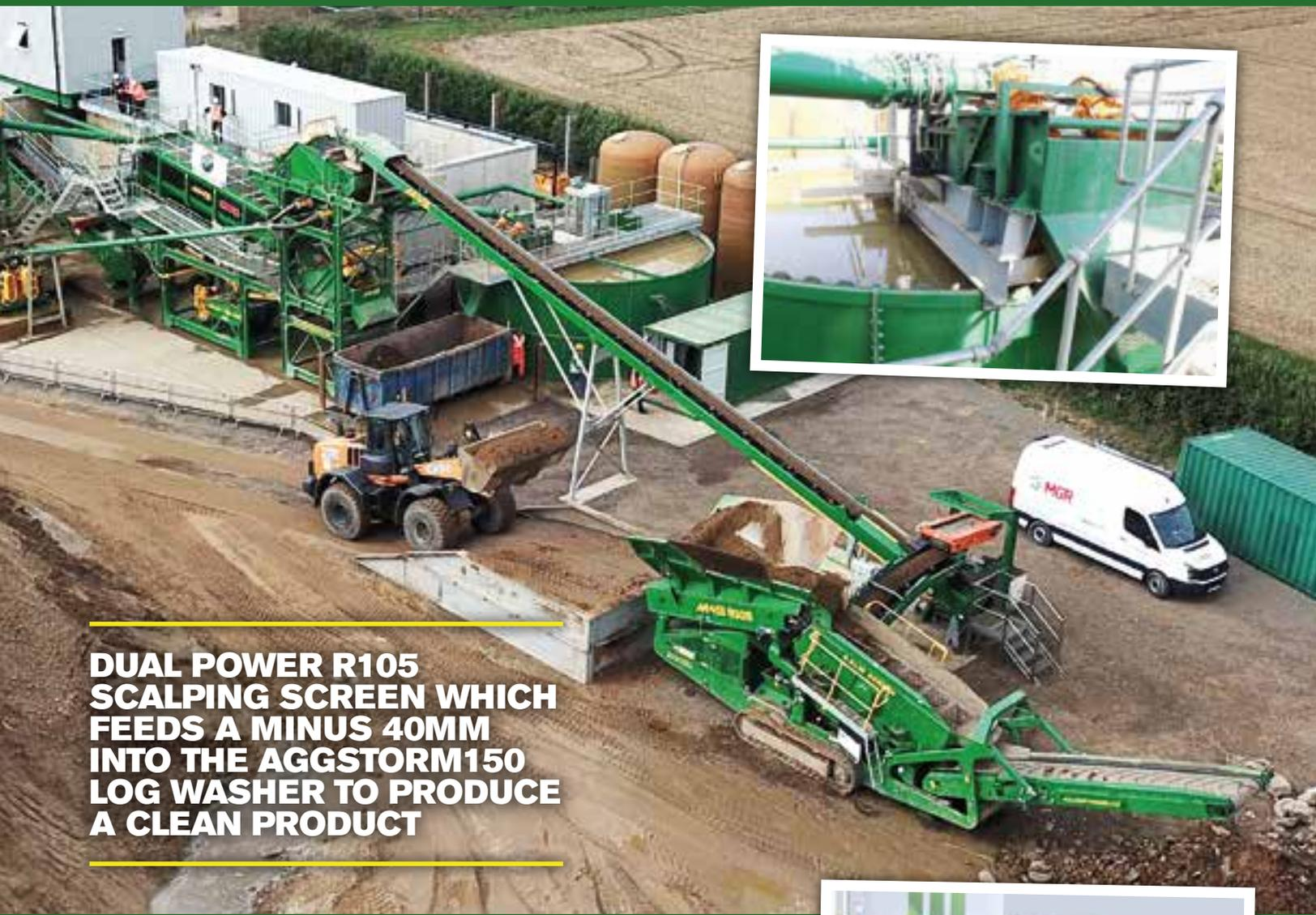
**DUAL POWER R105 SCALPING SCREEN WHICH FEEDS A MINUS 40MM INTO THE AGGSTORM150 LOG WASHER TO PRODUCE A CLEAN PRODUCT**
