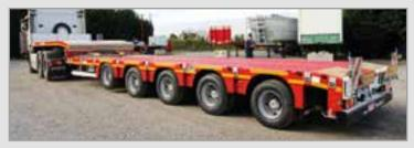
New Faymonville 5 axle step frame extendable low loader, 3 steeraxles, front lift axle, auto greaser, option on for hook on aluminium ramps or hydraulic ramps.
