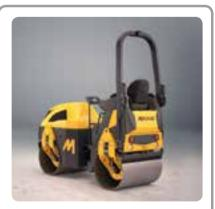
In 2018, *Mecalac* commenced a game-changing R&D project to redefine the compaction roller market. The result - its all-new TV1200 - this new concept is driven exclusively with a joystick on the right-hand side console. In removing the roller's steering column, Mecalac has revolutionised the access and driving style of this type of vehicle.
