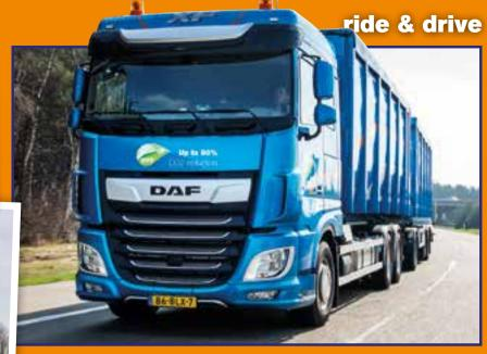
a tridem, consisting of the SR1360T tandem with single reduction or the HR1670T tandem with hub reduction, and a steered rearmost axle.
