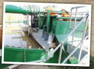
DUAL POWER R105 SCALPING SCREEN WHICH FEEDS A MINUS 40MM INTO THE AGGSTORM150 LOG WASHER TO PRODUCE A CLEAN PRODUCT
