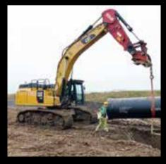
independent mechanical locking systems, ensuring both the front and rear attachment pins are locked in position preventing the attachment from accidental release.
