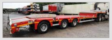
New 3 axle step frame low loader, extendable, with hook on aluminium loading ramps. 39ton payload, stake pockets an twistlock pockets.
