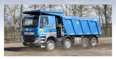
In addition to the existing 7.5, 8 and 9-tonne front axles, the new 10-tonne version in the CF and XF will be offered from the second half of this year. This is of particular interest for applications in the construction segment, where high front axle loads are commonplace.
