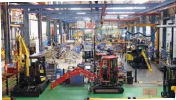
Yanmar's Saint-Dizier factory in France has one main assembly line capable of producing 25 machines a day.
