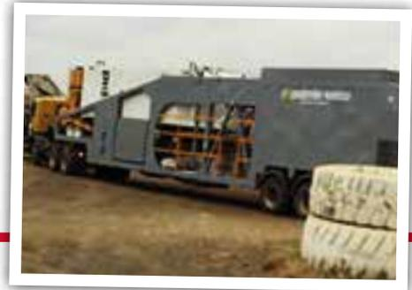
**Rapid International Ltd, based in County Armagh, has recently supplied Kasco Construction Ltd with a new Rapidmix mobile continuous concrete mixing plant for production of mine backfill within a mine in the North Mara region of Tanzania.**
