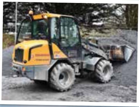
Due to its extra low front frame, this machine, powered by a 45hp Kubota V1505-T (4 cylinder) engine, can lift significantly more weight in comparison with its little 'brother' the V452T.
