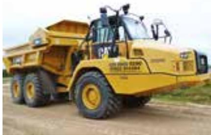
When it comes to productivity the Ejectors are much more efficient and ensure safer working on site. They're much more stable, and they're able to discharge whilst on the move or at inclines. In addition, operators are able to see the payload from the in-cab monitor. Quite simply, this means that operators can ensure the truck is neither under or overloaded, which has a direct impact on fuel burn per tonne on each cycle.
