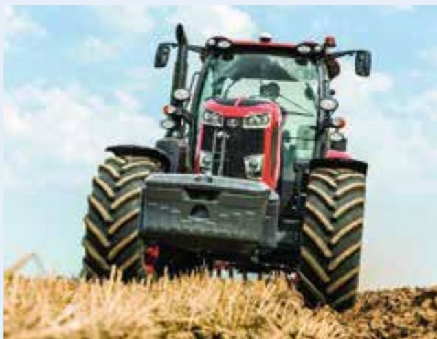
The main innovation in Kubota’s new M7002 Series is the new 6-speed Powershift transmission, which is either 30/15 or 54/27 if equipped with creeper. A number of its specifications have been improved, such as the increase
