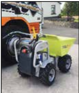
A Truxta B300-E zero emission Mini Dumper for CP Hire, from Ballyward Plant Services.
