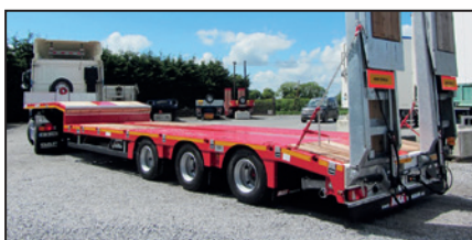
NEW Faymonville MAX 3 axle step frame low loader, 478ton gross, double flip ramps, rear steer axle
