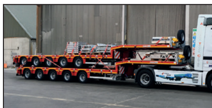
NEW Faymonville MAX 3 axle step frame low loader, 478ton gross, double flip ramps, rear steer axle
