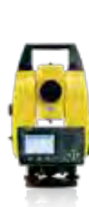
iCON builder 60 High-end manual total station, running iCON on colour touch screen.
