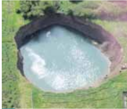
Large crown hole above abandoned salt mines near Carrickfergus in 2001
