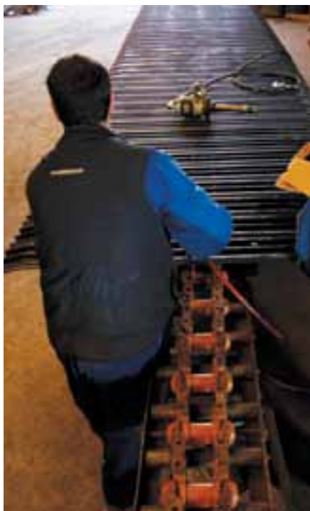
Fitting 1600mm Pads with Bent Ends to Track Chains
