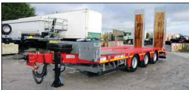
2016 New/Unused MAX 3 axle draw bar trailer, front lift axle, rear steer axle, 26ton payload, hydraulic ramps, out riggers, storage tray for out rigger timer, pockets for twistlocks. In stock ready to go.
