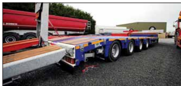
2016 New/Unused MAX 4 axle step frame low loader, front lift axle, two rear steer axles, out riggers, storage tray. Double flip ramps with side shift, greaser, 48ton payload. In stock ready to go.
