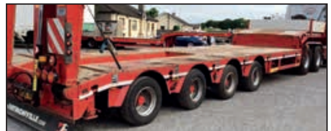
2007 Faymonville 4 axle 9ft wide step frame, fixed bed with trough, single ramps with hydraulic side shift, out riggers and steel rimmed timber, two rear steer axles, in test and ready to go straight to work.
