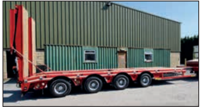
New Faymonville Heavy Duty 4 axle step frame low loader, extendable, trough, rear steer, front lift axle, double flip ramps, 13" out riggers, hydraulic legs under rear.
