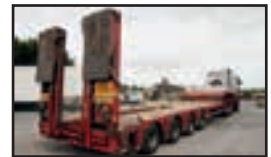
2007 Nootboom 4 axle 9ft wide step frame, 9.2m bed, trough, double flip ramps with side shift, two rear steer axles, out riggers, hydraulic suspension, in test, ready to go straight to work.
