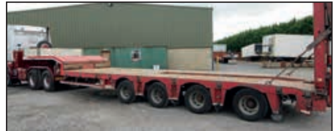
2007 Nootboom 4 axle 9ft wide step frame, 9.2m bed, trough, double flip ramps with side shift, two rear steer axles, out riggers, hydraulic suspension, in test, ready to go straight to work.
