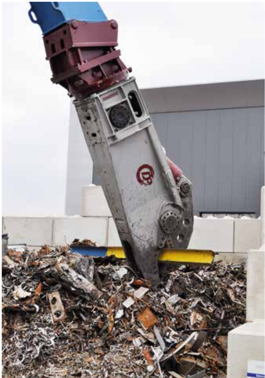
The DXS mobile Scrap Shear impresses with short operating cycles and a high closing force.
