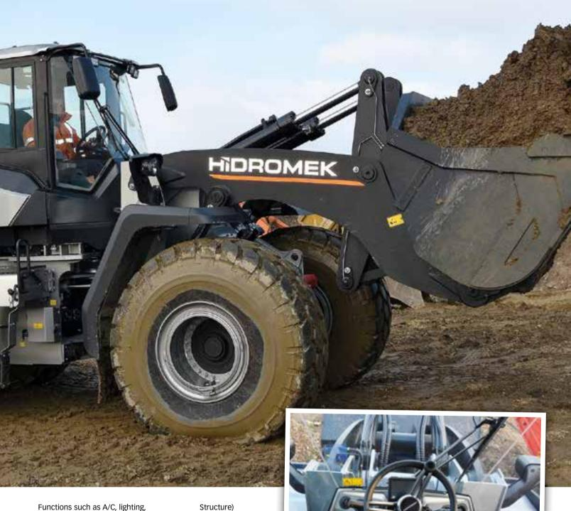
Functions such as A/C, lighting, radio, information display, etc. can be managed with the 8" high definition multimedia touchscreen which also serves as the display for the rear view camera when you shift to reverse. The steering, too, can be adjusted both telescopically and forward and reverse.
