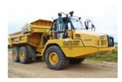
When it comes to productivity the Ejectors are much more efficient and ensure safer working on site. They're much more stable, and they're able to discharge whilst on the move or at inclines. In addition, operators are able to see the payload from the in-cab monitor. Quite simply, this means that operators can ensure the truck is neither under or overloaded, which has a direct impact on fuel burn per tonne on each cycle.
