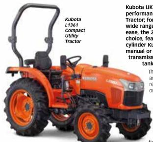
Kubota UK has launched its latest high performance L1361 Compact Utility Tractor; for those looking to complete a wide range of maintenances task with ease, the 36.6 HP machine is a flexible choice, featuring a powerful three cylinder Kubota D1803-M-E2 engine, manual or three range speed hydrostatic transmission and a 38 litre capacity fuel tank for extended periods of use.
