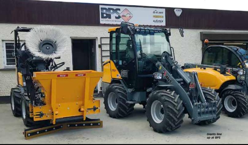
Due to its extra low front frame, this machine, powered by a 45hp Kubota V1505-T (4 cylinder) engine, can lift significantly more weight in comparison with its little 'brother' the V452T.
