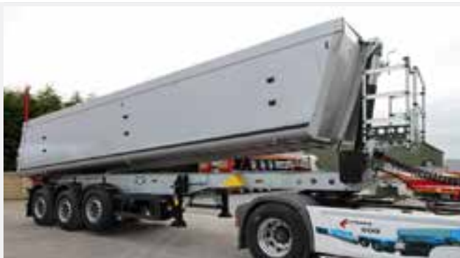
9.6m Aluminium Schmitz tipping trailer, Rear steer axle, auto dump on suspension, front lift axle, galvanised steel chassis, In Stock available now.
