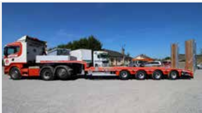
New 58ton gross Faymonville 4 axle step frame, fixed bed and extendable version, two rear steer axles, front lift axle, Double flip ramps, out riggers, ramps to neck, auto greaser. In stock available now.
