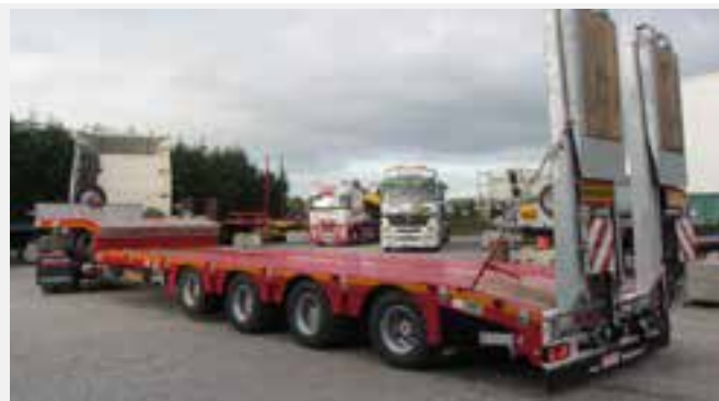
New 58ton gross Faymonville 4 axle step frame, fixed bed and extendable version, two rear steer axles, front lift axle, Double flip ramps, out riggers, ramps to neck, auto greaser. In stock available now.
