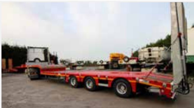
New 48ton Gross Faymonville 3 axle fixed bed low loader, rear steer axle, double flip ramps, out riggers, ramps to neck, storage trays, auto greaser, In Stock, available now.
