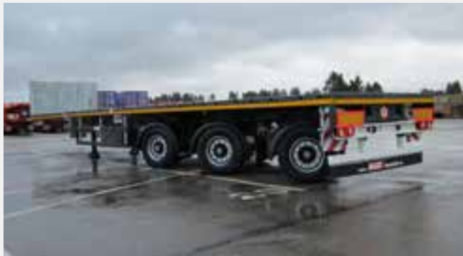
21m power steered extendable flat in stock, all 3 axles hydraulically steer, 37tonb payload, twistlocks, post sockets, extra lashing rings for load securing, XL Rated. In stock available now.
