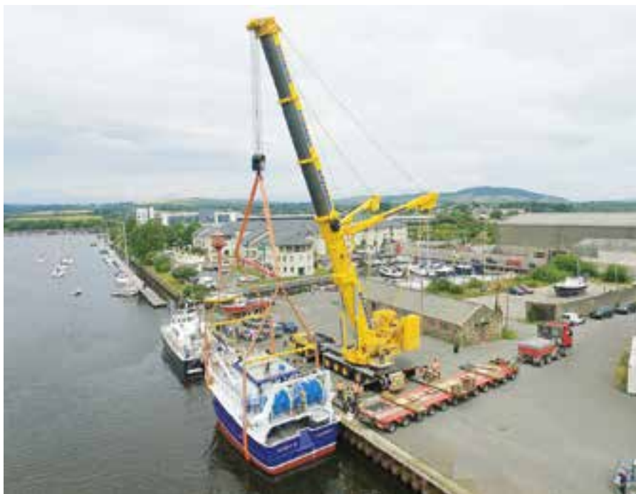
Kavanagh's LTM 1500-8.1 assisting with the launch of a 115 tonne fishing vessel, Diligent Jo, at Arklow Harbour, Co. Wicklow in Ireland.
